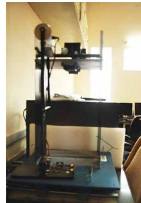
Automated Geosynthetic-Soil Interface Shear Test Apparatus
