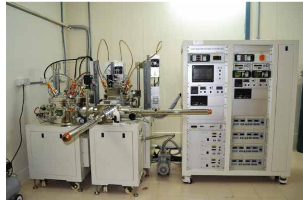
RF &amp; DC Magnetron Sputtering
