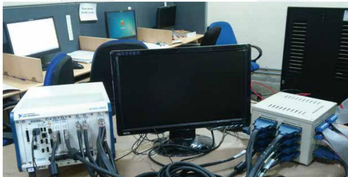
NI-PXIe-1062Q with Interface Module
