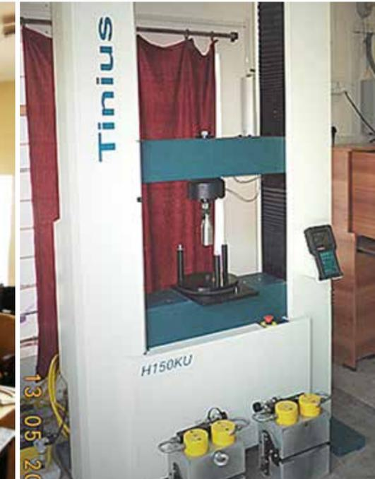
Geosynthetic Tensile Machine
