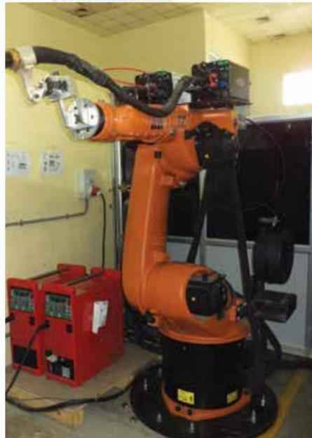
Robotic Welding Machine Twin-Wire
