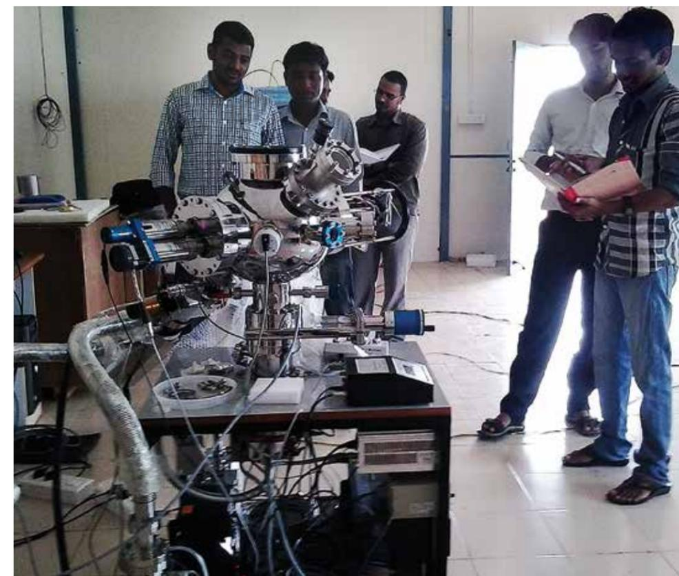
Pulsed laser deposition set up
