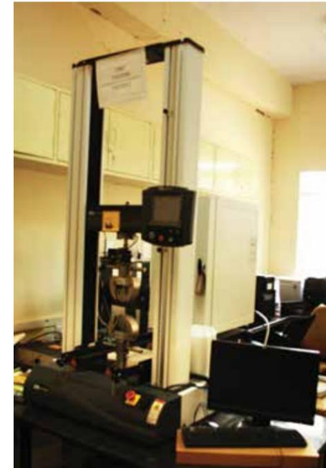
25KN UTM - Wire Testing Machine
