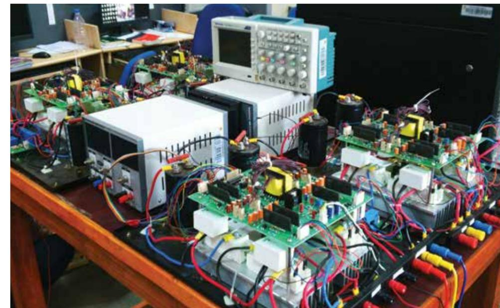
Multilevel inverter for Induction motor applications
